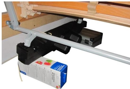
To remove the old motor first position a box or books under each end of the motor so it will only drop down a short distance. A stack of approximately 5" (13cm) is about right. This is about the only thing Yellow Pages are useful for. With the palm of your hand push down on the end of the motor and it should drop down. If it is tight give it a little bang but it should not need a lot of force.
