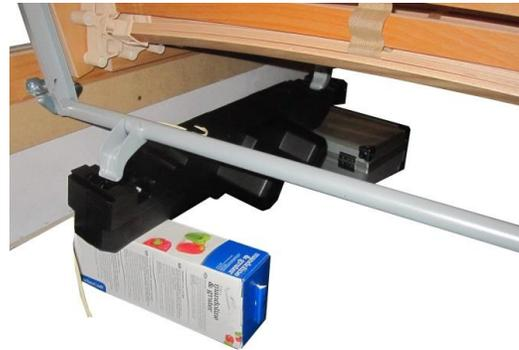
Manually lift the back section of the mechanism. It may stay up on it's own but it is safer to ask someone to hold it while you pass the new motor back inside the mechanism on top of the boxes in line with the hooks on the drive bars. Make sure you have the motors the right way around. There is an illustration on the motor to indicate the head and foot ends.
